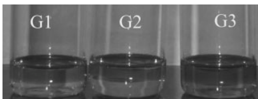
Figure 1 Photograph of chloroform (10 mL) solution of trapped Congo red by linear-dendritic copolymers (0.1 g dendrimer) at 25°C.
